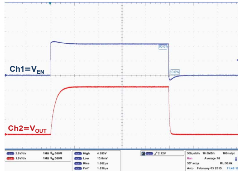
Figure 27. Startup with enable ( V_{OUT} = 3.3\text{ V} )
